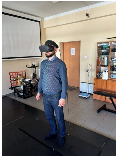
Figure 3. One of the participants in the experimental Vroom paradigm setup is standing on the Footscan system balance platform while donning a VR headset.
