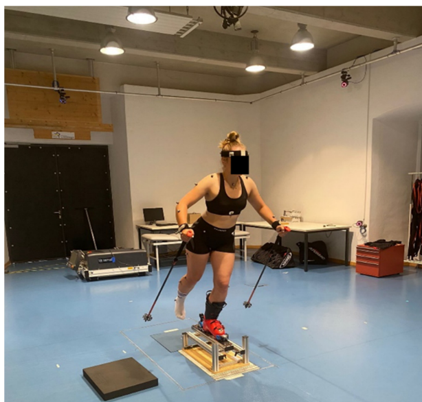
Figure 1. Full-Body-Plug-in Gait marker setup used in the study.
